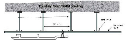
STEP 1 Position & screw-tightened the ceiling strip
